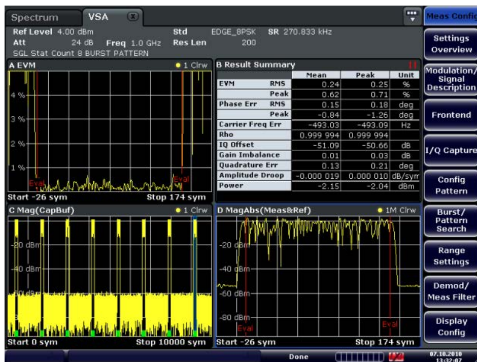
Fig. 8-10: Result range that exceeds the burst length
