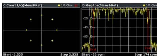
Fig. 8-11: Evaluation lines properly adjusted
