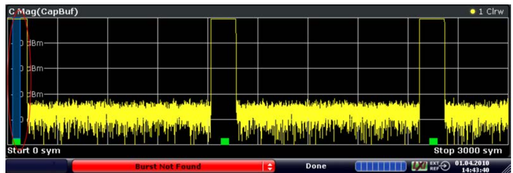
Fig. 9-3: Example for measurement on incomplete burst capture
